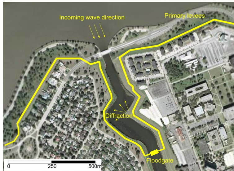
Figure 5.16: Location of the floodgate. The shape of the canal outlet will cause diffraction of incoming waves. Image from: Google Earth [11].
