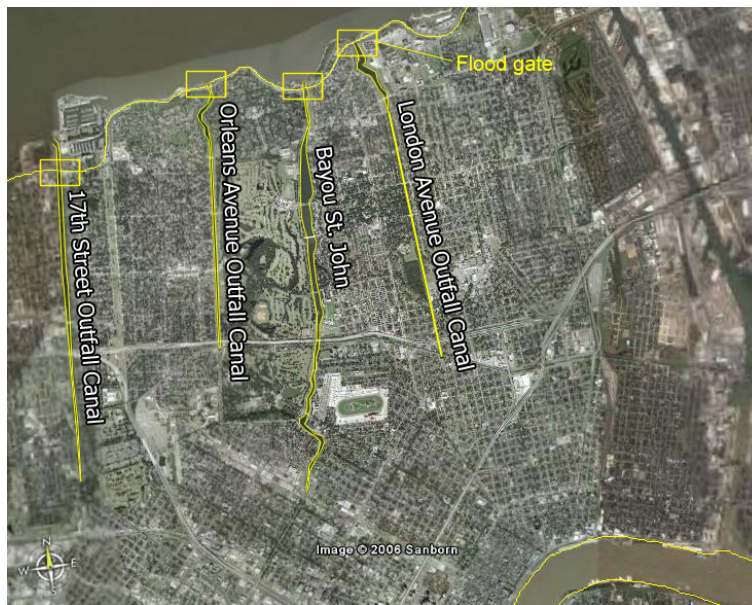
Figure 5.11: Closing the canals with floodgates can significantly reduce the length of flood defenses. Image from: Google Earth [11].
