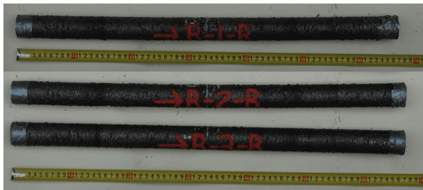
Figure 4.38: The specimen shape after buckling lab test.
