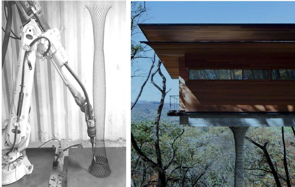
Figure 2.13: AM diagrid column [35]. (Left: The manufacturing of AM diagrid column, Right: The application of the diagrid column as a tree-house support.)
