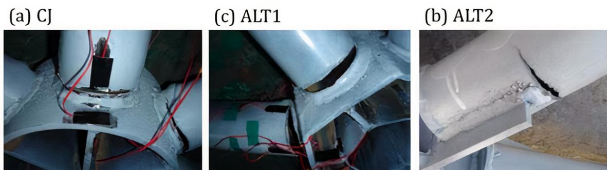
Figure 2.27: Failure modes of joints. (a). CJ, (b). ALT1, (c). ALT2 [49].
