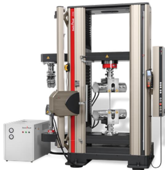
Figure 3.8: Tensile test setup (machine: Zwick/Roell Z250).
