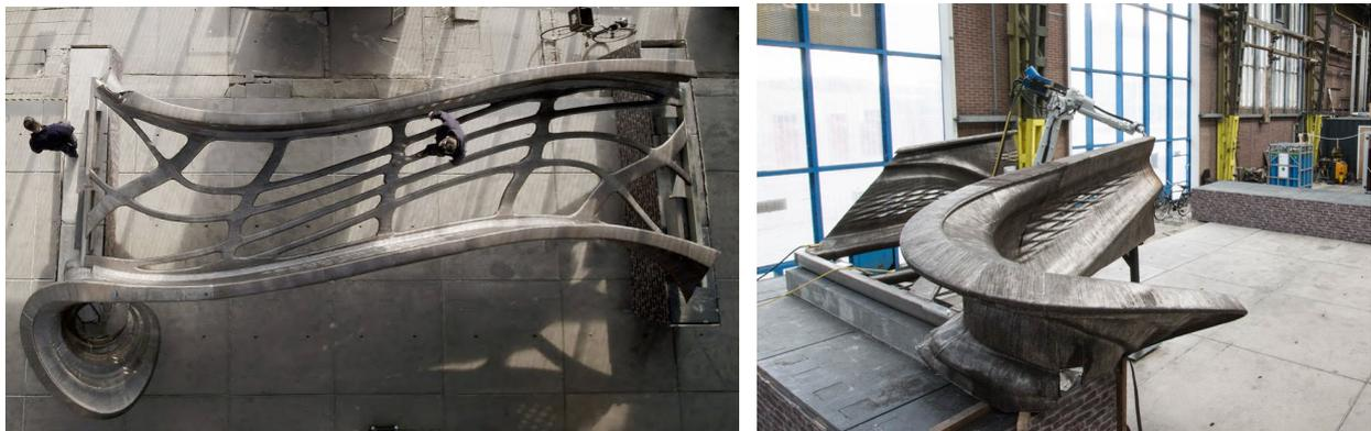
Figure 2.14: MX3D AM (WAAM) bridge. (Left: Overview of the bridge; Right: The bridge under printing.)
