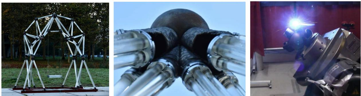
Figure 2.12: TU Delft glass swing. Left: The overview of the glass swing; Middle: The most complicated node in the swing (the top node), and Right: The rotatory table for printing a node.
