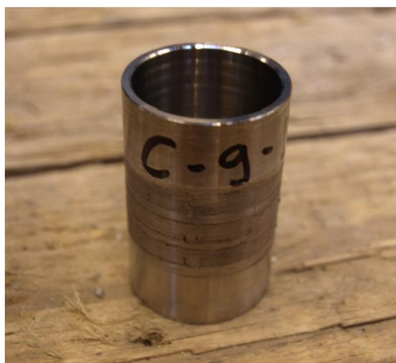
Figure 3.10: The compression test specimen.
