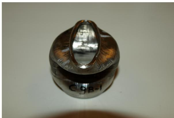
Figure 4.20: The Compression lab test failure.
