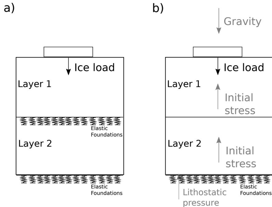
**Figure 1.** Schematic of a) the EF, and b) the NG model approaches. In grey are the forces and stresses specific to the NG approach.
