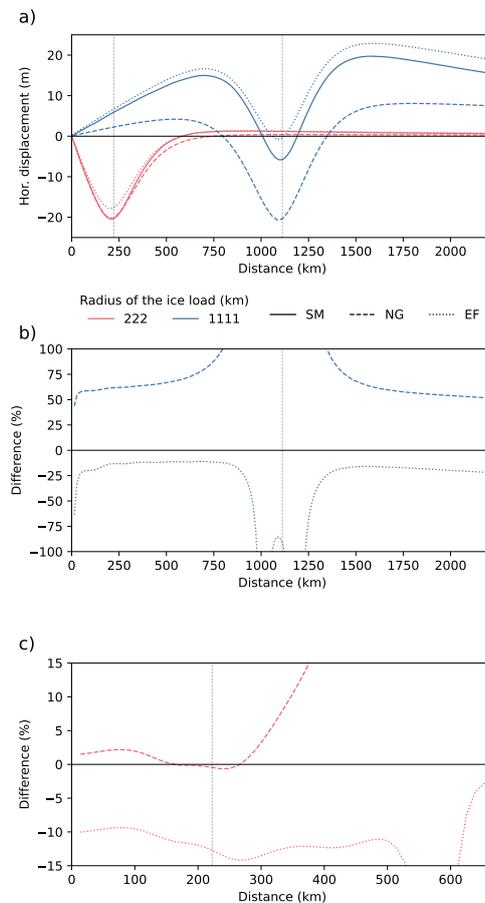
**Figure 5.** (a) Horizontal displacement after 10 ka of loading using ice loads 1,111 and 222 km in radius for SM, NG, and EF, as well as the difference of NG and EF with SM for (b) the 1,111 km and (c) 222 km radius ice sheets. The edges of the ice loads are marked by vertical grey dashed lines.
