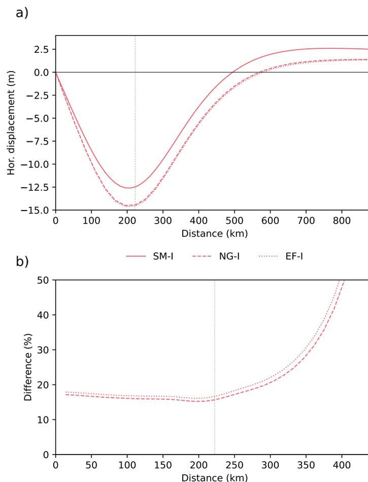
**Figure 3.** a) Horizontal displacement after 10 ka of loading as simulated by SM-I, NG-I, and EF-I, and b) the difference of NG-I and EF-I with SM-I. The dashed and dotted lines are on top of each other in Figure a. The edge of the ice load is marked by a vertical grey dashed line.
