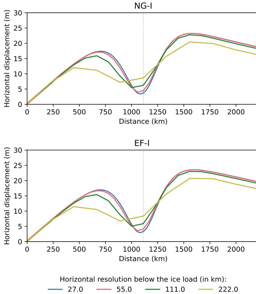
**Figure S6.** Difference in horizontal displacement after 10ka of loading for NG-I (a) and EF-I (b) due to changing the horizontal resolution below the load, for the 1111 km radius disc load.
