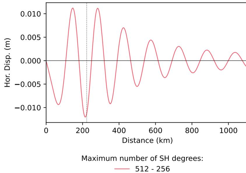
**Figure S1.** Difference in modelled horizontal displacement after 10ka of loading with a disc load 222 km in radius.
