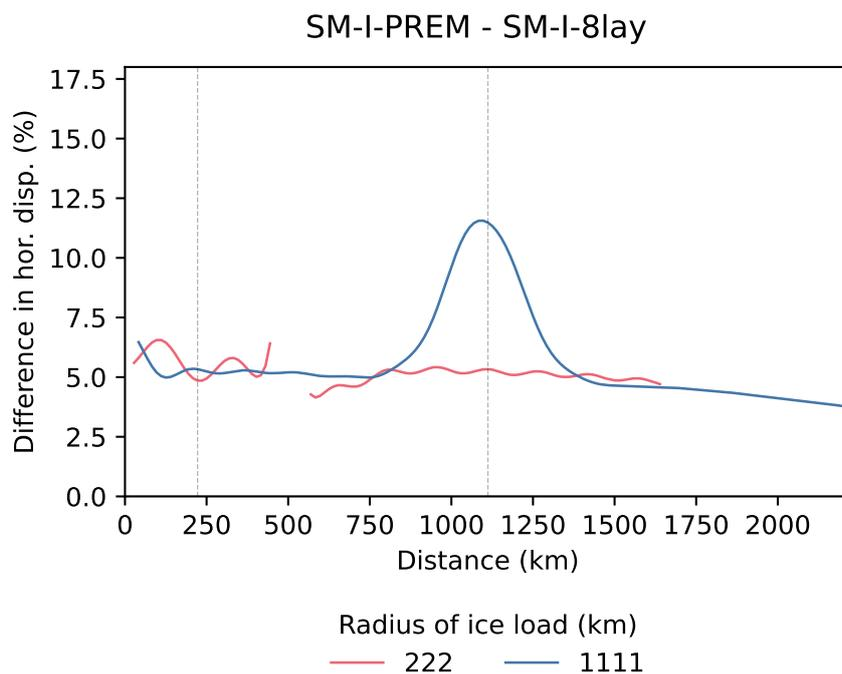
**Figure S3.** Difference in horizontal displacement due to the Earth model approximation for the incompressible ICEAGE model, using 10 ka of loading. When the absolute value of the original signal is below 1.5m, the values are masked.
