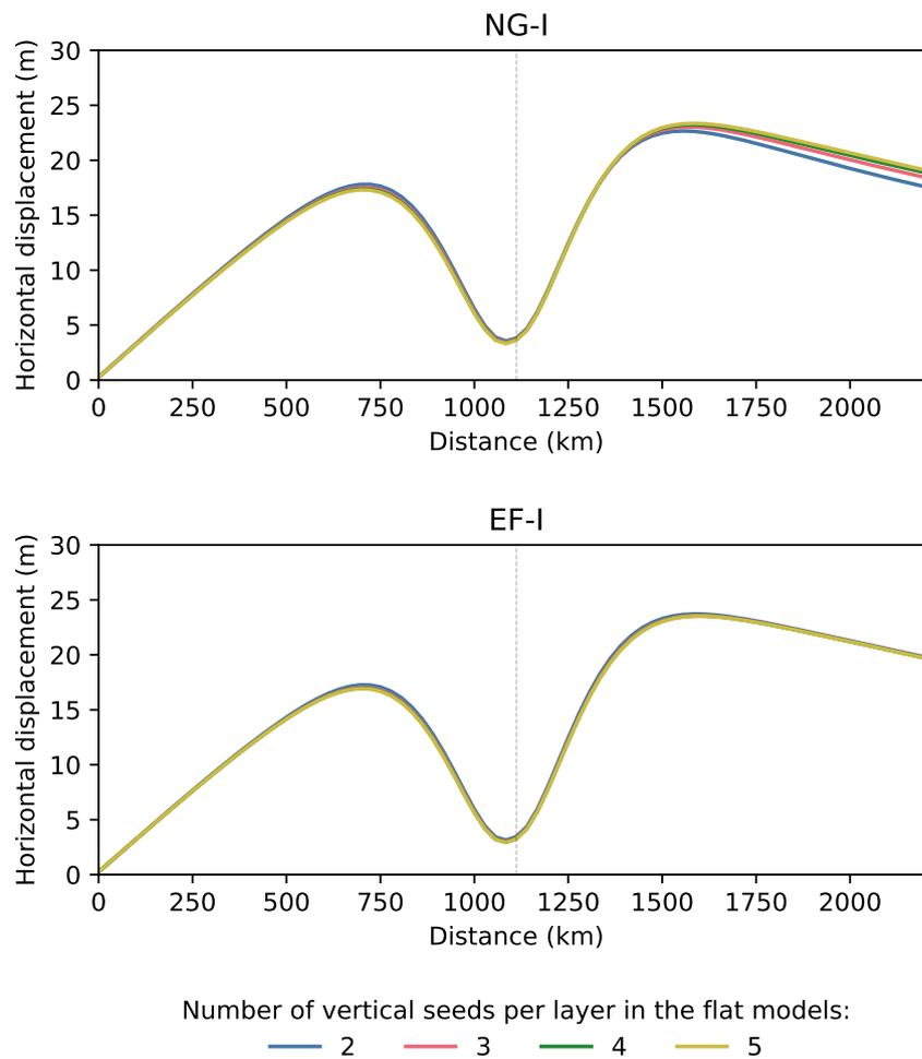
**Figure S5.** Difference in horizontal displacement after 10ka of loading for NG-I (a) and EF-I (b) due to changing the amount of elements per layer, for the 1111 km radius disc load.
