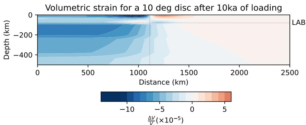
**Figure S7.** Volumetric strain after 10ka of loading with a 10 deg disc in box-NG. Positive values denote compression, and negative values dilatation. The Lithosphere-Asthenosphere Boundary (LAB) is denoted by the horizontal dashed line.
