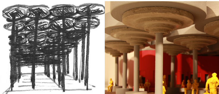
Figure 3.21: what started as a rough design sketch ended up being cast in actual concrete in the 1:50 scale model.
