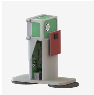
(a) Concept casing for the system with magnets
