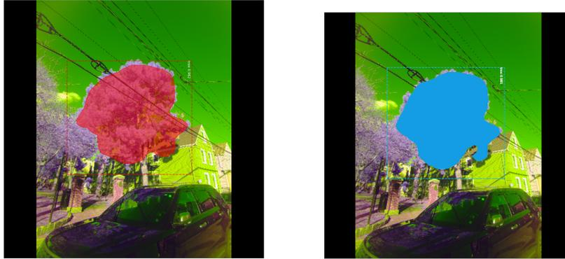
(a) Segmentation output from Mask R-CNN using full Tensorflow model
