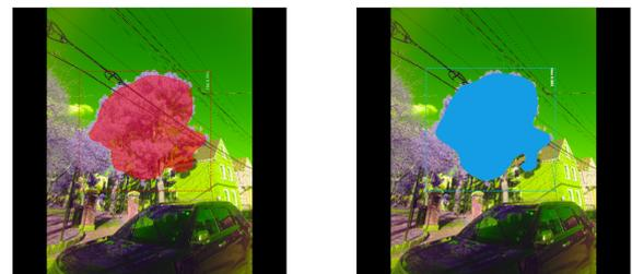
(a) Segmentation output from Mask R-CNN using full Tensorflow model (b) Segmentation output from Mask R-CNN using Tensorflow-lite (quantized)
