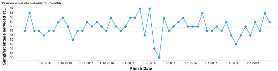
Figure 26: Percentage of train units of the full fleet worked on at all Service Locations on all Mondays
