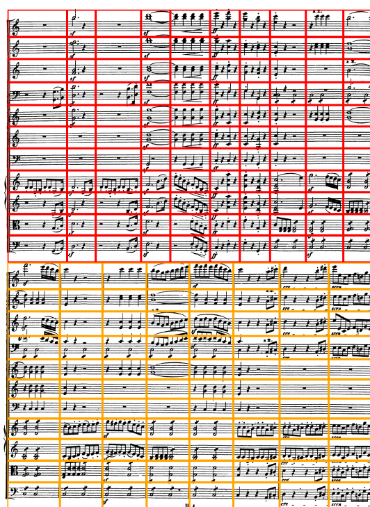
Figure 6.2: Boundaries of each measure on an example page. These boundaries are where the images for each individual measure will be cut off.
