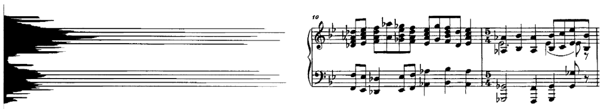
Figure 2.1: An example of horizontal projection of a small excerpt of music. The stafflines create clear peaks in the histogram. These are figures 11 and 10 from Bainbridge et al. [1], respectively.
