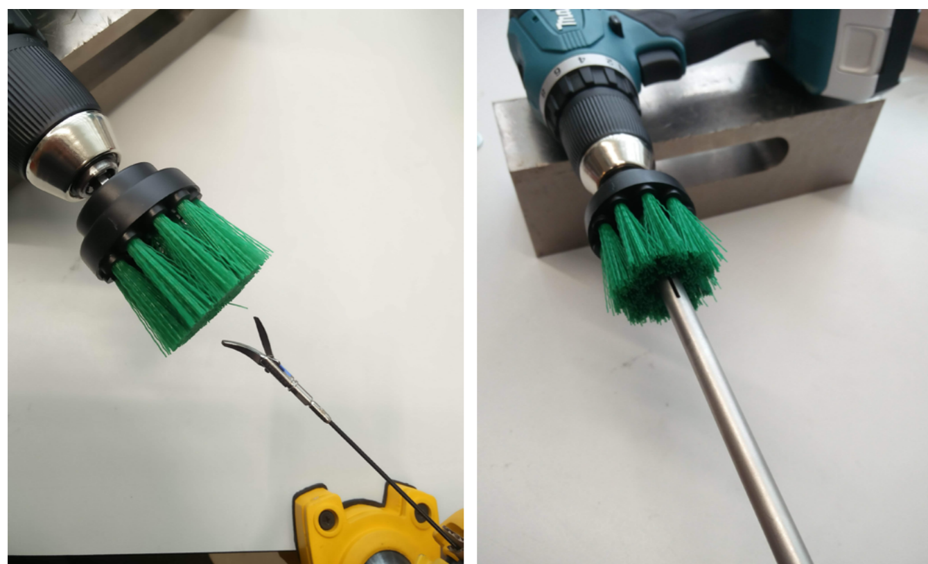
Fig G.4.2 Testing a single rotary drill brush with a a flexible non lumened grasper insert (left) and a 10mm diameter lumened clip applicator (right).
