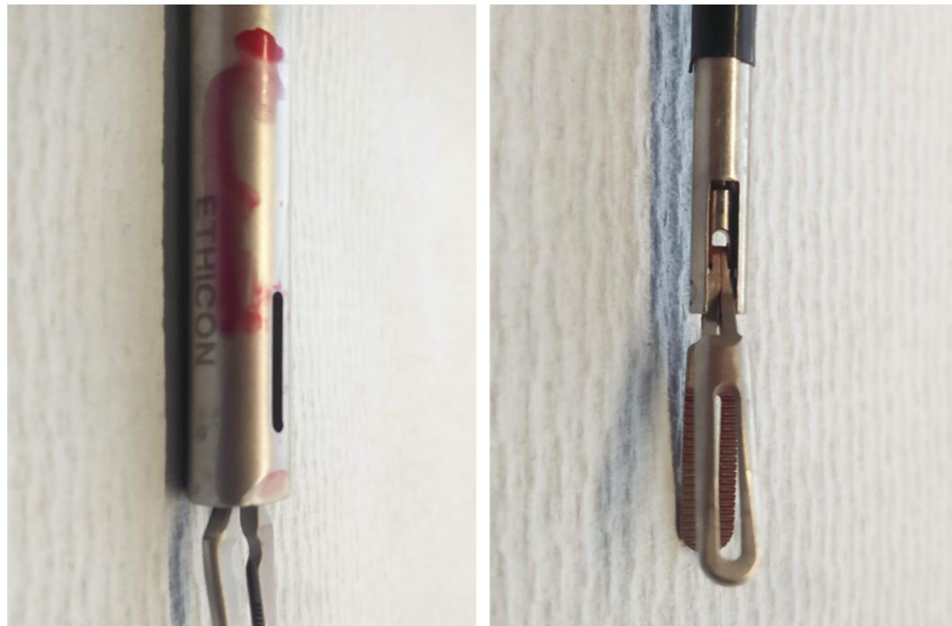
Fig G.3.2 Residual contaminants visible to the naked eye after testing in this setup.
