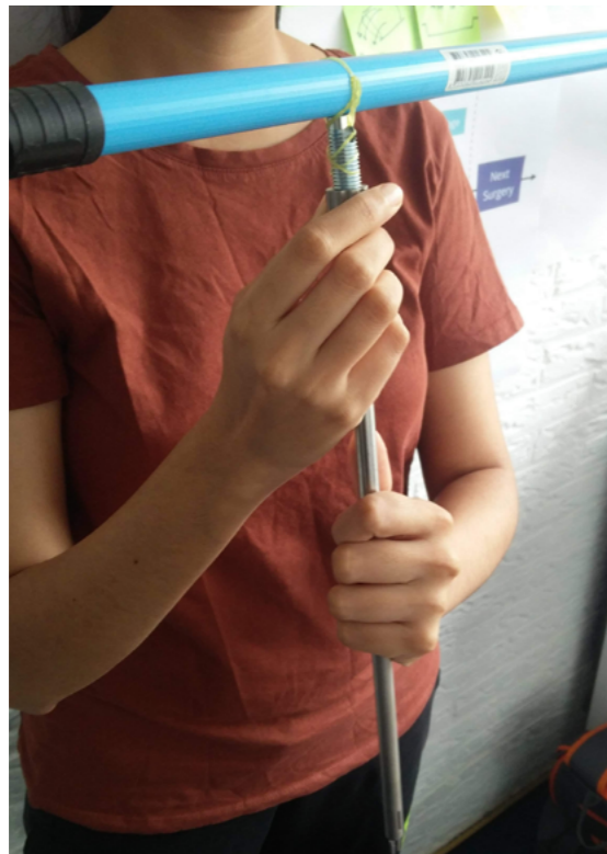
Fig G.2.3 Attaching the laparoscopic instrument to a make-shift luer lock nozzle. Participant uses both hands to support the instrument.
