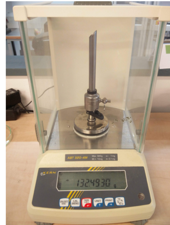
Fig 1. Microgram scale used to measure slight variations in the surgical instrument weight.
