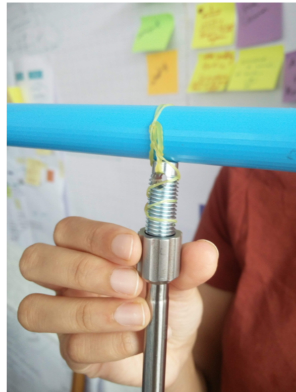
Fig G.2.4 Turning the threading of the laparoscopic instrument to the make-shift luer lock nozzle. Participant had trouble aligning the threading to the nozzle.
