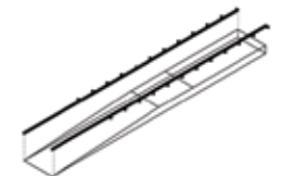
Hand rail requirements 900mm - 1000m m
