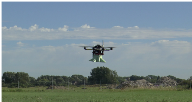
Figure 4.1: MavTec MAV flying outdoors with the DVS128 event based camera attached.
