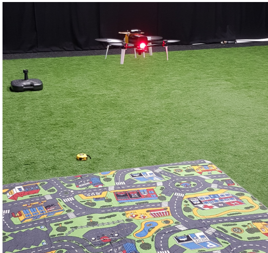
Figure 5.2: Parrot Bebop 2 quadrotor MAV equipped with SEEM1 Dynamic Vision Sensor.
