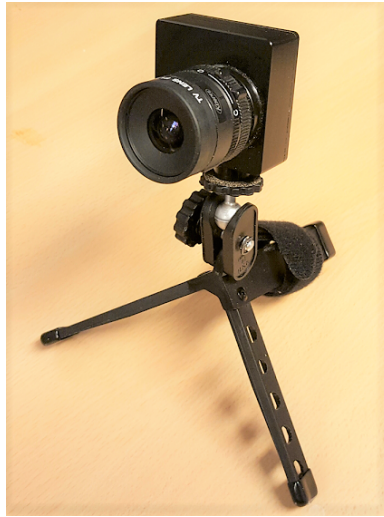
Figure 4.3: Picture of the event-based camera employed in this work, the DVS128.
