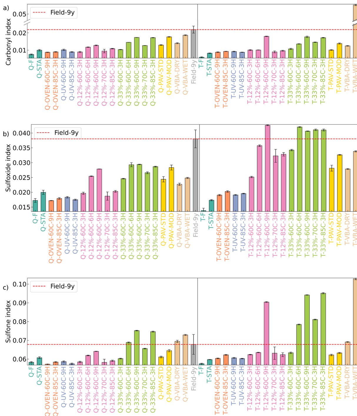
Fig. 2. FTIR indices of Q and T binders at different aging conditions summarized in Table 2: a) carbonyl index, b) sulfoxide index, c) sulfone index, d) hydroxyl index, e) aromatic index, f) aliphatic index, and long chain indices in the range of g) 710–734 \text{cm}^{-1} , h) 734–783 \text{cm}^{-1} , i) 783–833 \text{cm}^{-1} , j) 833–912 \text{cm}^{-1} .
