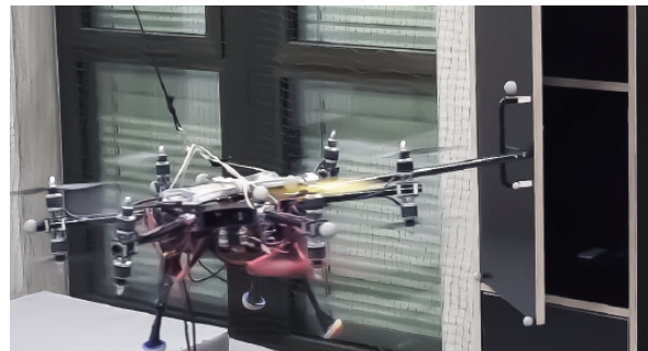
Figure 4.2: Fully actuated drone platform - with 6 independently tiltable rotors [7]
