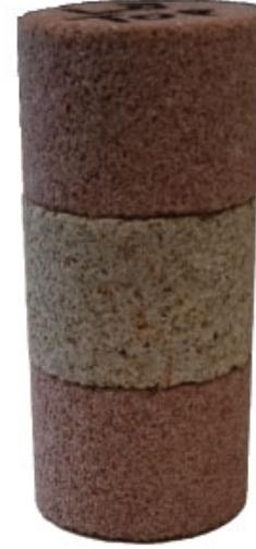
(a) Schematic overview of a synthetically layered sample. L1 refers to layer 1, L2 to layer 2, L3 to layer 3.
