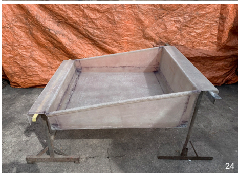
Phot. 15-24 GFRP water basin. Author's photography.
