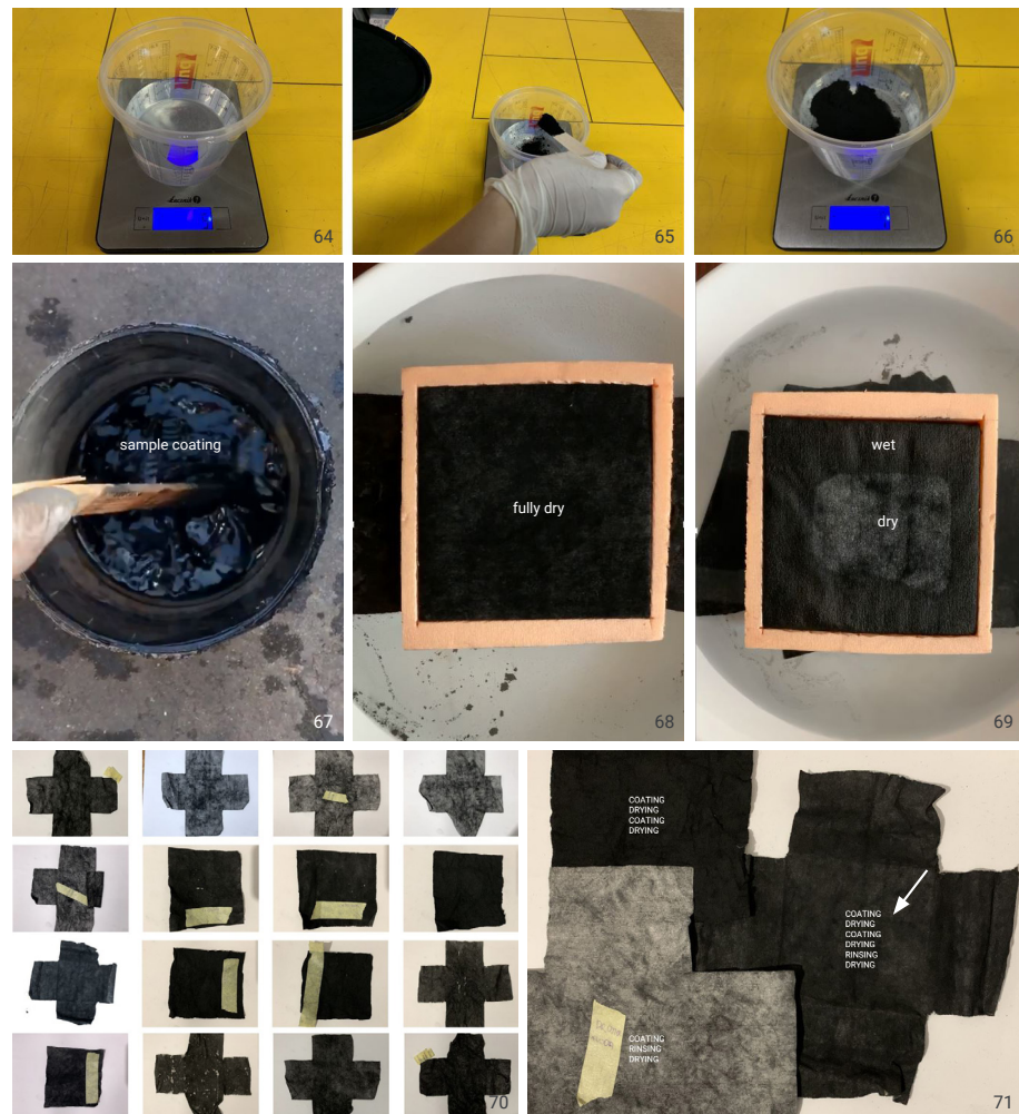
Phot. 64-71 Wipes coating test. Author's photography.
