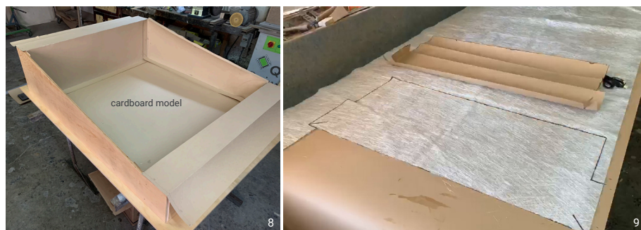
Phot. 8-9 Fiberglass mat cutting. Author's photography.
