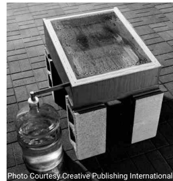
Fig. 15 Solar-based water purification methods. Author's graphics. Data source: (Luzi, Tobler, Suter, & Meierhofer, 2016; Saidur et al, 2011)
