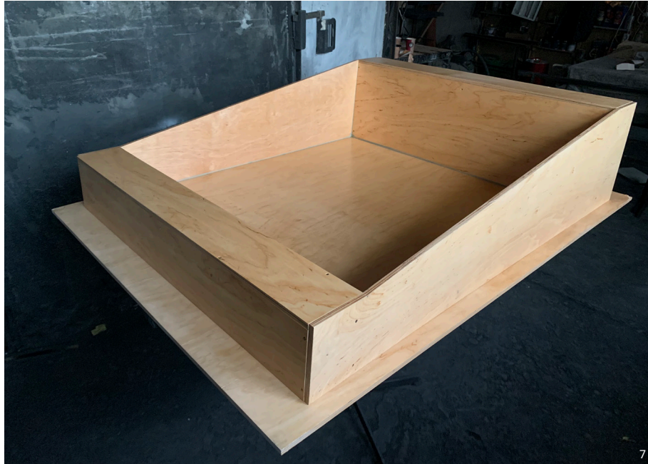
Phot. 7 Plywood mold covered with transparent lacquer. Author's photography.
