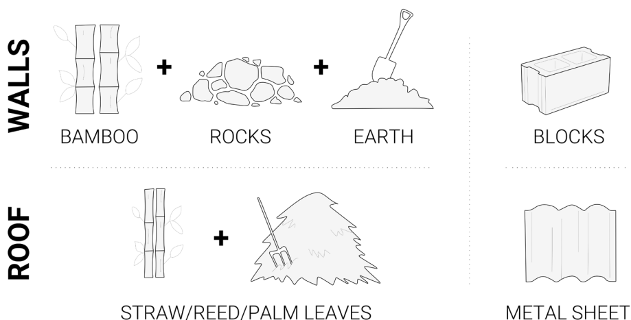
Fig. 37 Construction materials used in Beira region. Author's graphics.
