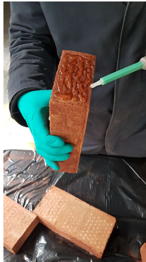
(b) T=1:32, applying adhesive;
