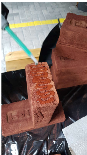
(a) T=14:58:45, applying adhesive;
