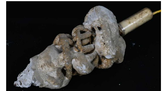
Figure 2.05 Starting and final structure after 4 months of growth in marine environment (Own pictures, 2026)
