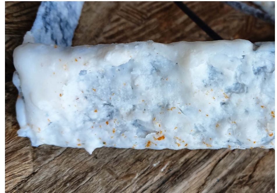
Figure 1.15 Biorock on steel cathode after one week of growth (Own picture)
