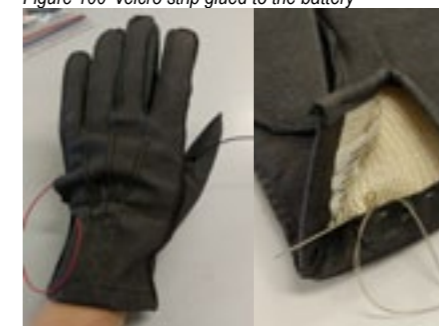
Figure 101 Openings to reach the wires
