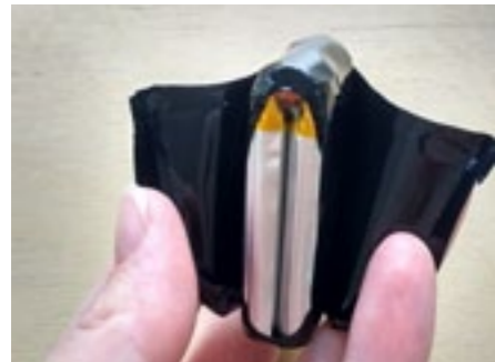
Figure 56 Battery pack 3.7 V contains two lithium polymer batteries
