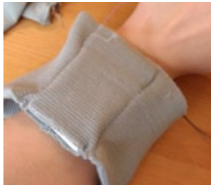
Figure 172 First attempt at stitching the elastic band inside
