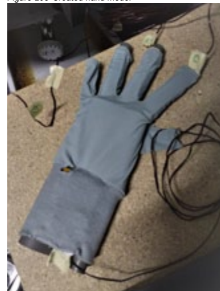
Figure 206 Placement of hand model and thermometer probes C1, C2, C3 and C4.
