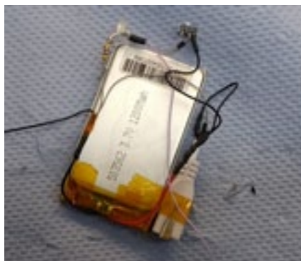
Figure 189 Low voltage connector connected to the other components in parallel
