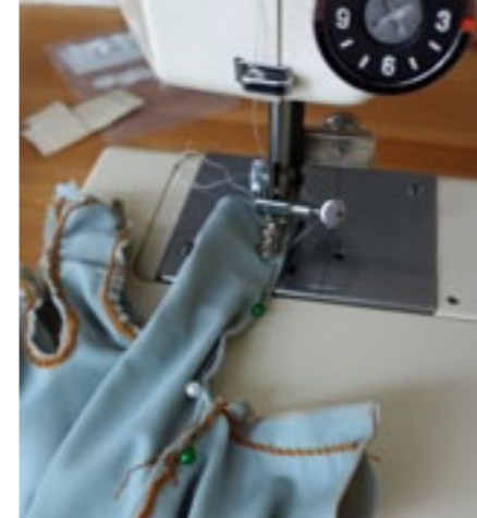
Figure 166 Sewing the resistive wire at the index finger with an all-purpose thread straight stitch
