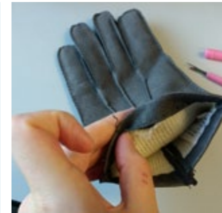
Figure 99 Opening up the seam of the lining
