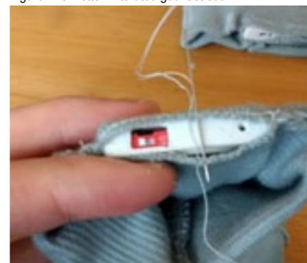
Figure 177 Handstitching the battery pack into place
