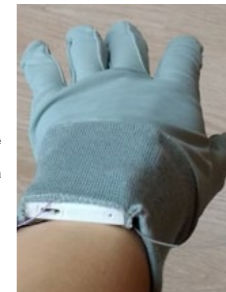
Figure 182 Switch and LED facing the user at the short end of the battery pack
