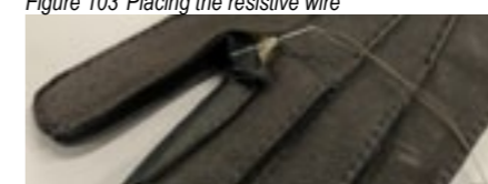
Figure 103 Placing the resistive wire
