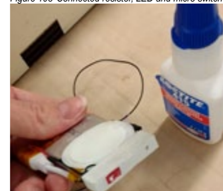
Figure 195 Gluing the cover on battery pack 2
