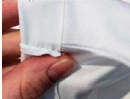
Figure 162 Serafil 1 mm zigzag stitch on a pattern iteration model
