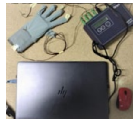
Figure 208 Test setup. Laptop, SquirrelSQ800 with K-Type thermocouples and inner glove prototype.
