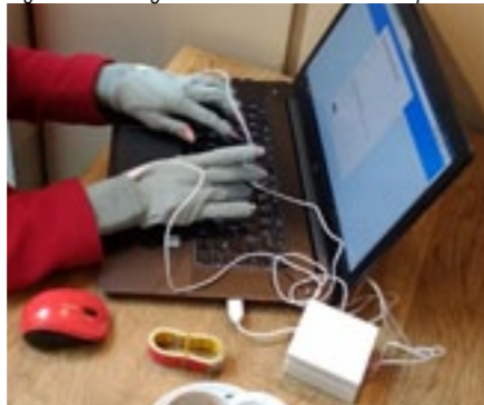
Figure 201 Prototype charger in use, connected to the inner glove prototypes
