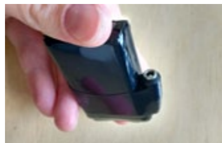
Figure 57 Battery pack with low voltage connector
