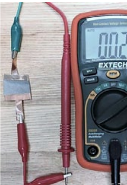
Figure 78 Lowering the resistance of conductive fabric by connecting it over the entire length
