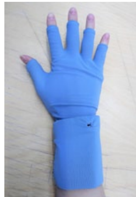
Figure 143 Gauntlet test using the wide elastic band covered with elastomer. A ridge is formed at the wrist.
