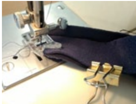
Figure 163 Gütemann all-purpose thread 1 mm zigzag stitch on outer glove prototype
