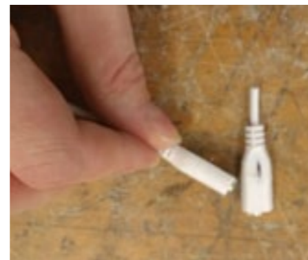
Figure 190 Low voltage connector sanded down to match the battery thickness
