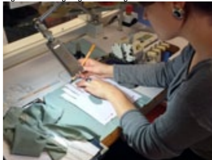
Figure 153 Linda tracing the basic glove pattern on the elastomer to create the first version of the inner glove
