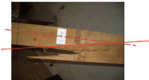
Figure 5: Bending failure of a tropical hardwood beam initiated by the presence of global slope of grain.
