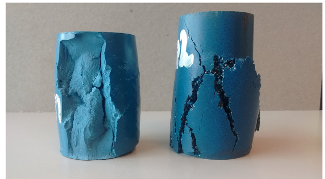
Fig. 12. Typical failure modes for resin (left) and steel-reinforced resin (right).
