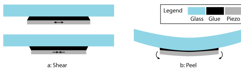
Figure C.3: Schematic representation of the glass-glue-piezo assembly, stressing the need for (a) high shear strength and (b) high peel strength.
