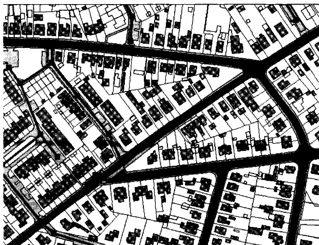
Figure 43: An example of the result of applying GIS techniques for obtaining information with respect to amount and type of surfaces contributing to run-off generation. Different shades of grey indicate different types of surface. A technique like e.g. Thiessen polygons (also known as Dirichet tiles or Sobolov spaces) is used to assign individual surfaces to the manholes at which they are supposed to discharge under storm conditions.
