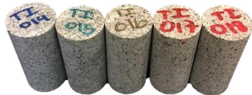
Figure 9 Eifel basalt cores (left) and Benin granite cores (right)
