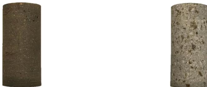
Figure 33 Dark color basaltic andesite Tangkuban Perahu (left) and light color andesite Tangkuban Perahu (right)
