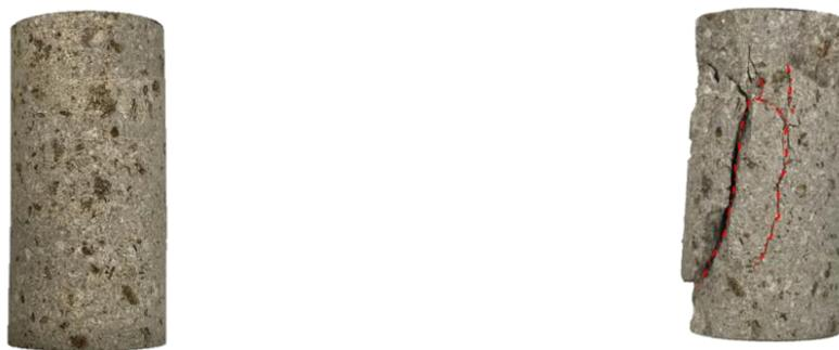
Figure 40 Andesite Tangkuban Perahu core before UCS test (left) and after UCS test (right)
