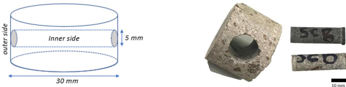
Figure 14 Small size core illustration (left) and small size cores from Tangkuban Perahu heated at  $500^{\circ}\text{C}$  (right)
