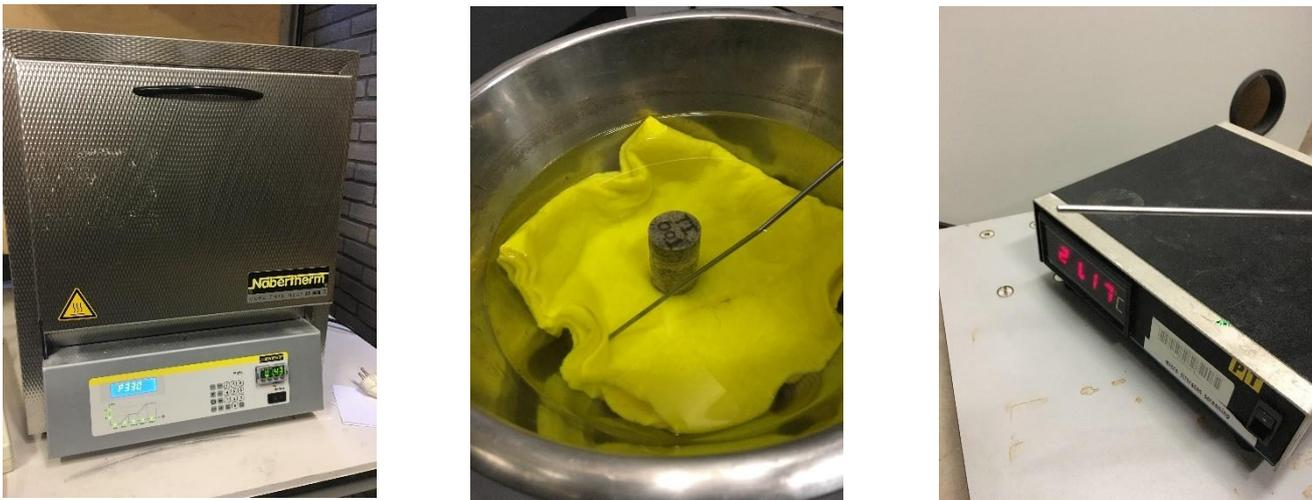
Figure 15 Oven to heat the cores (left), thermal shock creation process (middle), temperature sensor (right)
