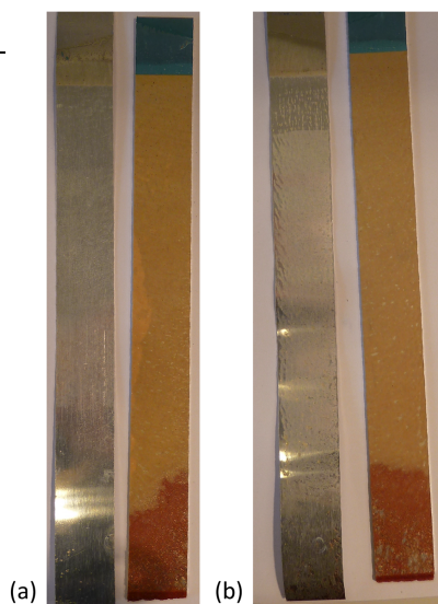
Figure 7: Visual images of peeled panels bonded with Redux 775 after PAA RT (a) and PAA 50°C (b). The peeled area starting a few centimeters below the blue tape was first peeled under dry- and then wet conditions.
