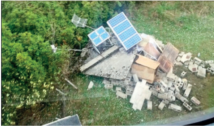
◀ Figure 2, Damaged French GPS station GUMB; neither the GPS receiver nor the antenna was harmed (image courtesy: John Galetzka).
