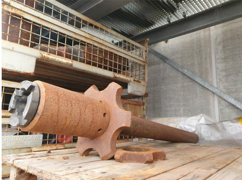
Figure B.2: Push core used at the RCSG location
