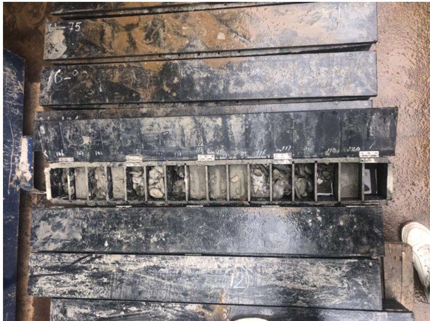
Figure B.3: Sample bin in Rotterdam showing big clay lumps
