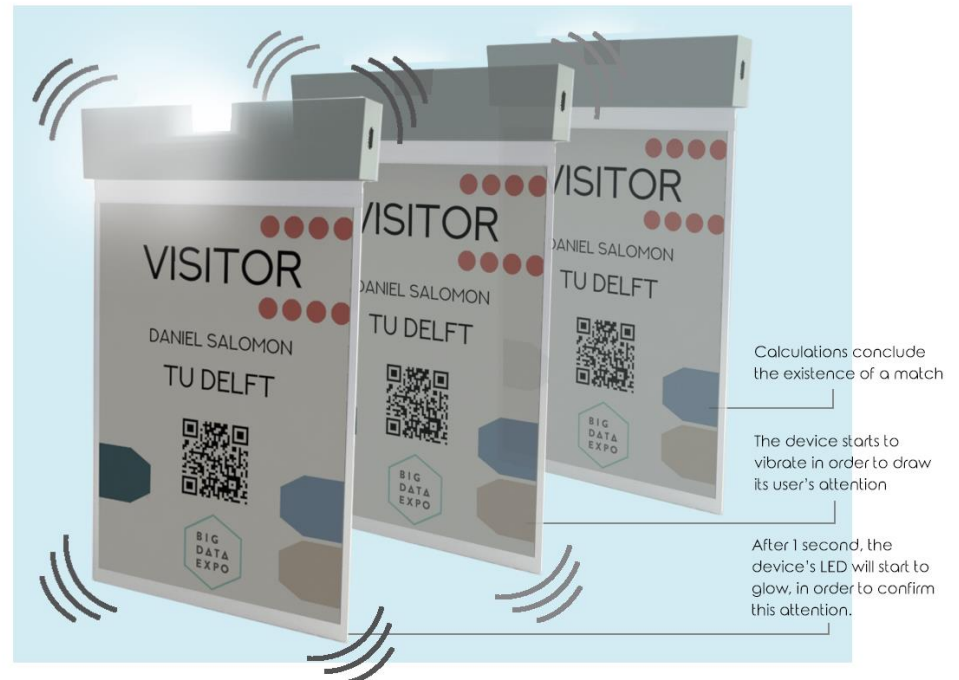
Figure 31: The personal device's nudging process
