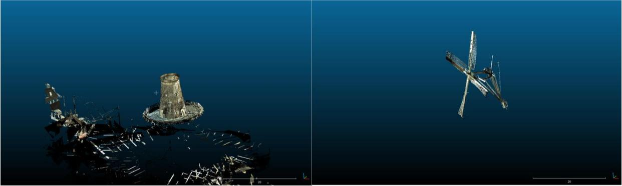
Figure 23 & 24: cutting balcony in parts (resp. 36 million and about 4.5 million points)
