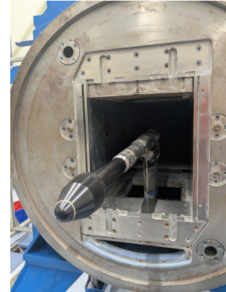
Figure 3.6: WT model with trip strip on the nose
