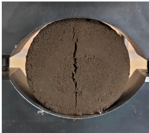
(a) Tensile Crack observed in one of the tests.
