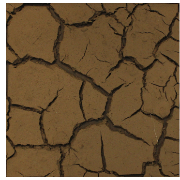
(c) Final crack pattern for SP-9.2 from March 2025.
