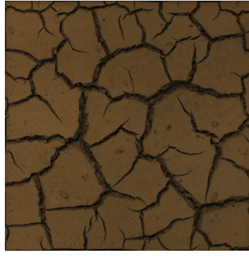
(b) Final crack pattern for SP-9.2 from September 2024.
