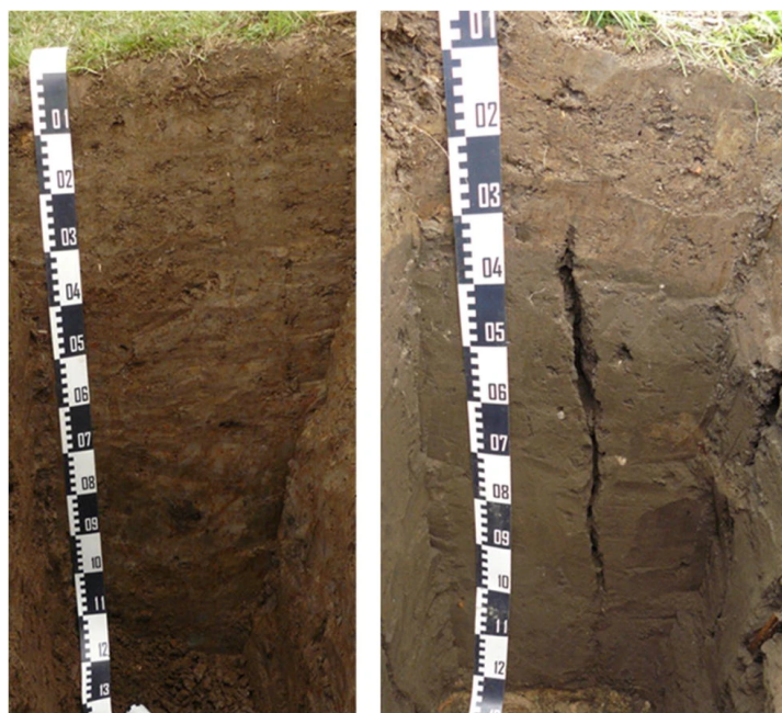
Figure 2.13: Profile view of the cover layer built with marsh sediments (left) and dredged materials (right)[29]
