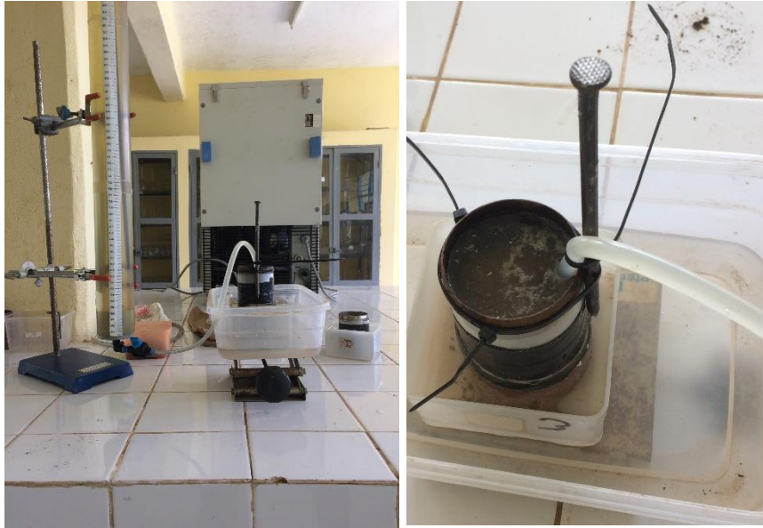
Figure 4.4: Saturated permeability set-up in laboratory (left) and close-up of sample being tested (right)
