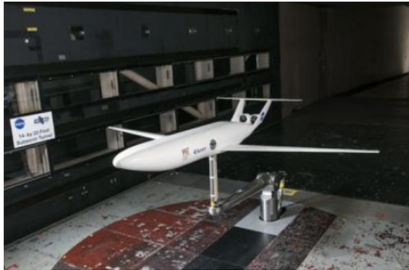
**Figure 2.5:** A model of the D8 configuration in the NASA Langley's wind tunnel. [13]
