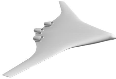
**Figure 2.4:** A render of the Blended Wing Body concept with boundary layer ingesting turbofan engines. [11]
