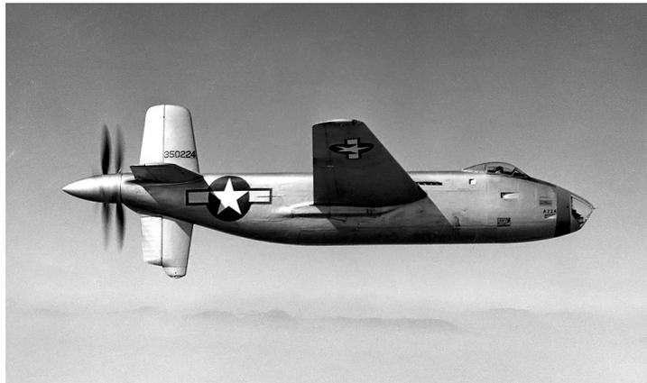
**Figure 2.3:** An early example of an aircraft utilizing BLI was the Douglas XB-42, which conducted its first flight in 1944. Picture taken from Wikimedia Commons<sup>2</sup>.
