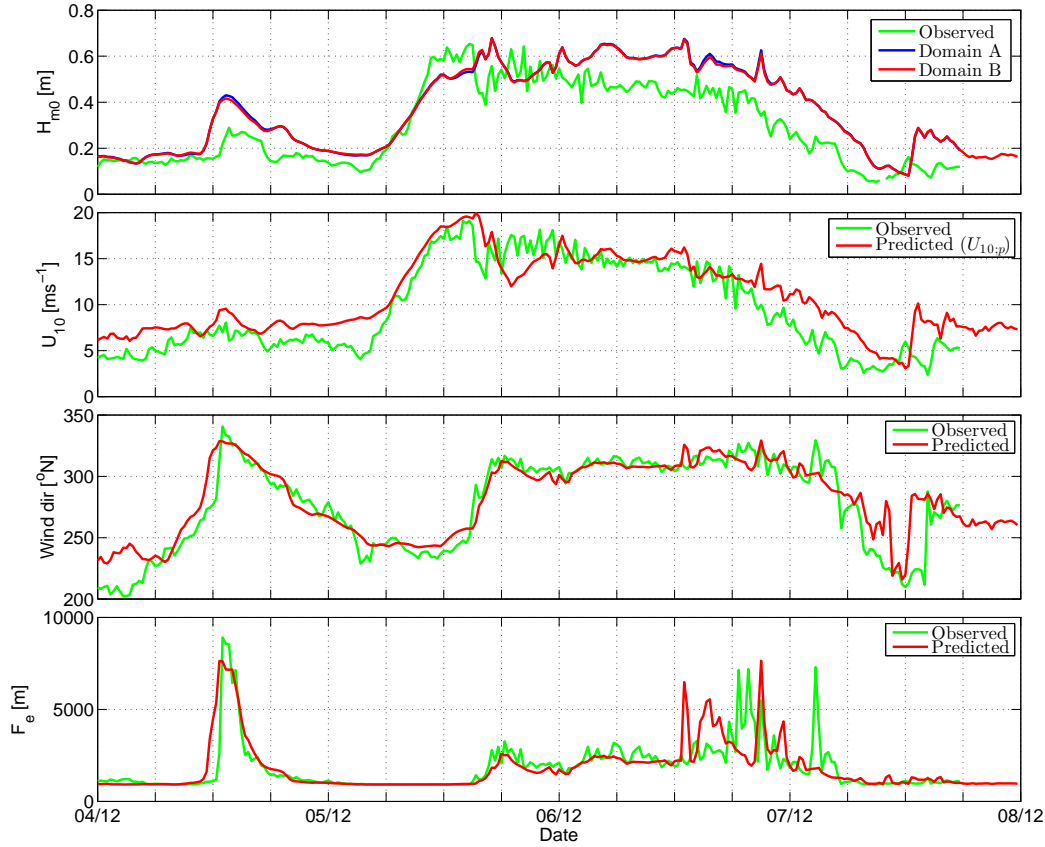
Figure 5.5: Storm 2: Significant Wave height ( H_{m0} ), (Pseudo) Wind Speeds ( u_{10;p} ), Wind direction ( \theta_{\text{wind}} ), and the Effective fetch ( F_e )
