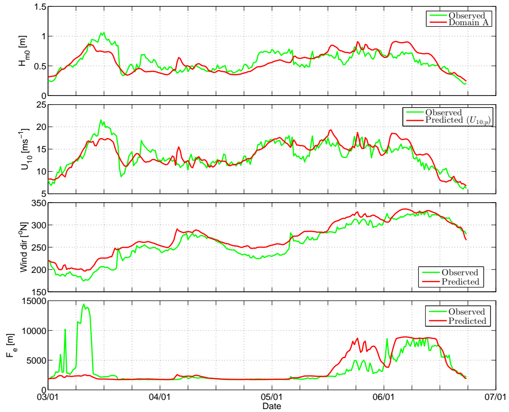
Figure 5.4: Storm 1: Significant Wave height ( H_{m0} ), (Pseudo) Wind Speeds ( u_{10;p} ), Wind direction ( \theta_{wind} ), and the Effective fetch ( F_e )
