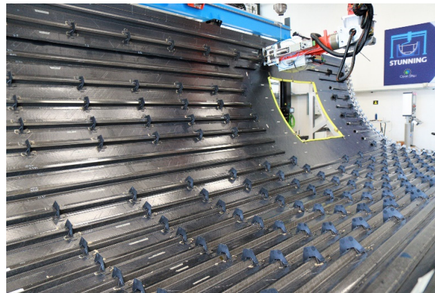
Figure 14. The lower shell of the MFFD demonstrator after welding the clips to the skin and stringer.
