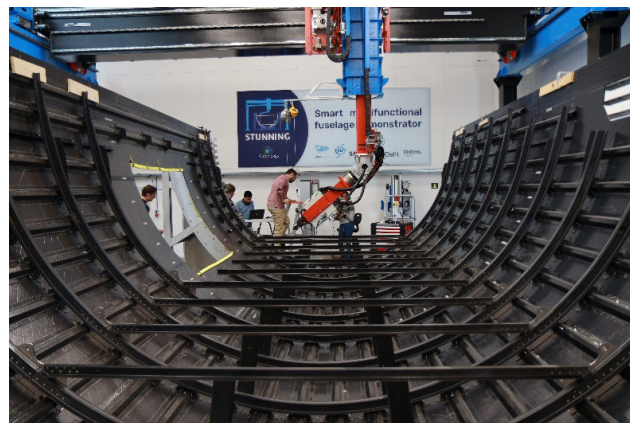
Figure 15. The lower shell of the MFFD demonstrator after welding the frames to the clips.
