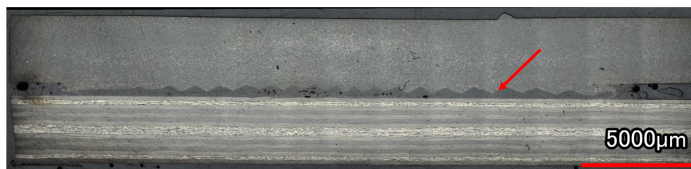
Figure 16. Cross-sectional micrograph of welded joint between clip (upper part) and flat skin panel (lower part) with 2 shim layers. Red arrow indicates the weld line, which exhibits partially intact energy director ridges and a resin-rich area between the clip and skin panel.
