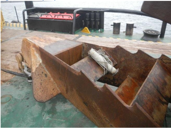
Figure 8 picture of the anchor with the wave logger
