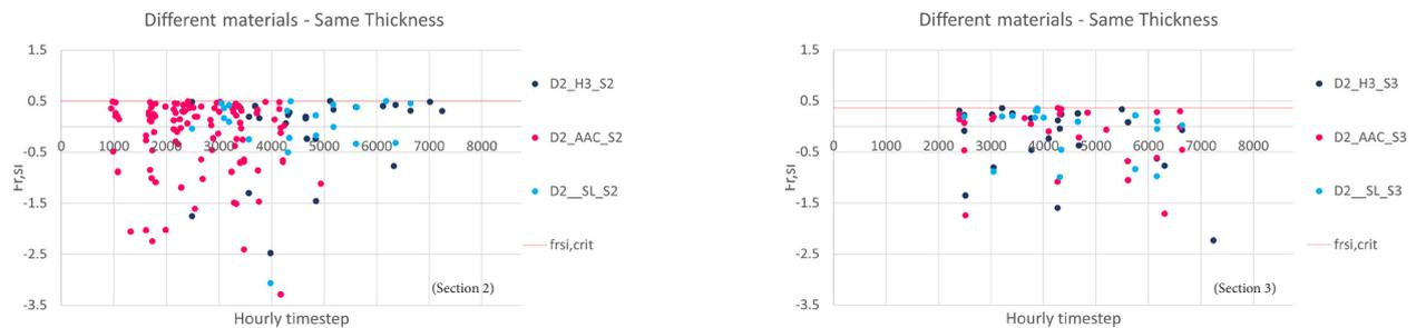
(b): The surface condensation - Comparison between the materials (same thickness) - Detail 2
