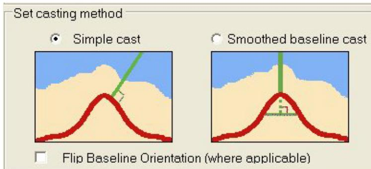
the transect lines is of importance and influences your results. When using the smoothing tool, the program doesn't draw a line perpendicular at that specific place, but it draws the transect perpendicular to a line between two points on the baseline. This
