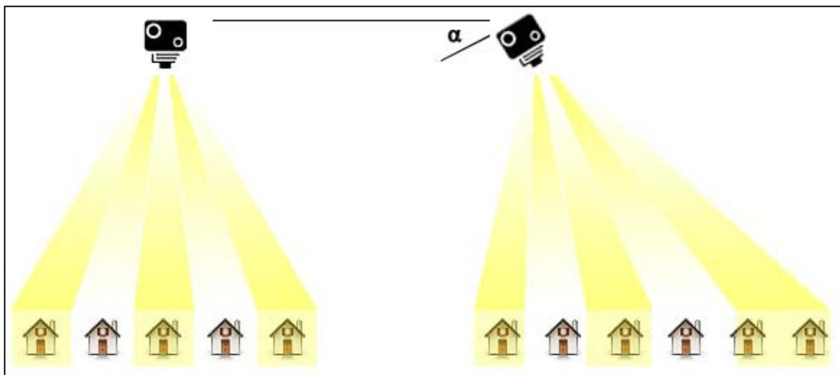
**Figure A-8 Introduction of errors in aerial photographs due to tilting of the camera with respect to the earth surface**
