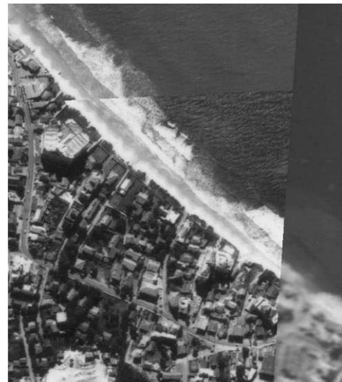
**Figure A-10 Blurred at edges and errors due to composition [Project Ingleses 2007]**
