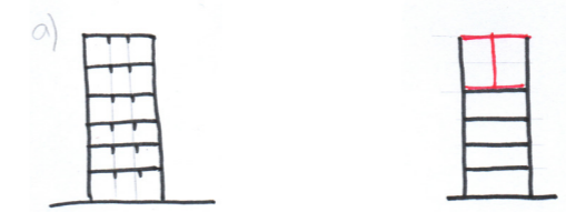
a) Demolish top level & add ultra-lightweight structure
