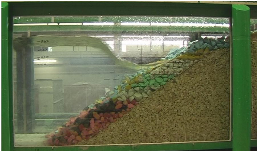
Figure 3.3 A view from the video camera, setup S03TM, H_s = 0.12\text{m}
