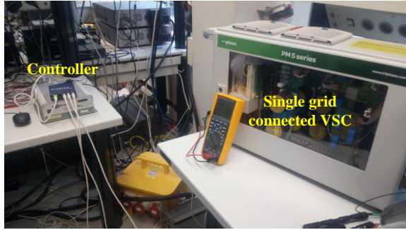
Figure 6.14: Two-level VSC Triphase/PM5F30C used for experimental validation.
