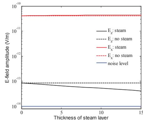
Figure 3: Thickness of steam layer and the corresponding vertical and horizontal electric field amplitudes for the Schoonebeek model with increasing steam thickness at a source-receiver offset of 4 km.
