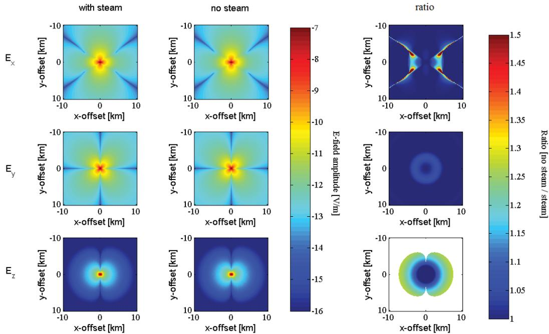
Figure 2: Electric field amplitudes for the model from Figure 1 with a 5 m thick steam layer inside the reservoir (left column) and without steam layer (central column), and corresponding field ratios (right column), for a frequency of 0.5 Hz. Field ratios are not shown where amplitudes are below  $10^{-14}$  V/m.  $E_x$  (a – c),  $E_y$  (d – f) and  $E_z$  (g – i) receivers are located at a depth of 100 m, and an x-directed point source is assumed.
