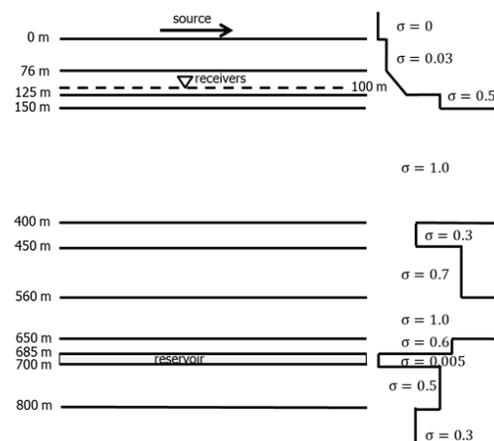
Figure 1: Layer model and conductivity profile (in S/m) derived from logging data. The source represented by the black arrow is placed at the surface, and receivers are placed at a depth of 100 m.
