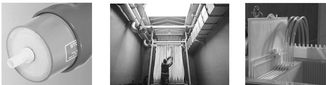
**Figure 5: picture of (a) a tubular membrane (b) hollow fibre membrane (c) flat sheet membrane**
