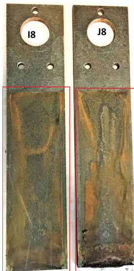
(a) Corroded steel plate I8 and J8 of specimen with a crevice of 10mm height and 150mm long. (The exposed area is indicated by the red box.)
