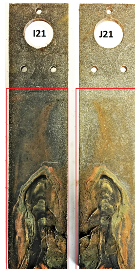
(b) Corroded steel plate I21 and J21 of specimen with a crevice of 2mm height and 150mm long. (The exposed area is indicated by the red box.)
