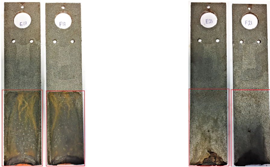
(a) Corroded steel plate E17 and F17 of specimen with a crevice of 4mm height and 100mm long. (The exposed area is indicated by the red box.)
