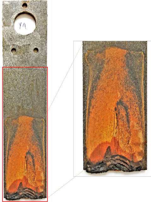
Figure 5.36: Corroded steel plate Y4 of a specimen with a 4mm high crevice and a 14mm high void.
