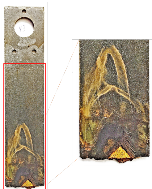
Figure 5.35: Corroded steel plate Y1 of a specimen with a 2mm high crevice and a 14mm high void.
