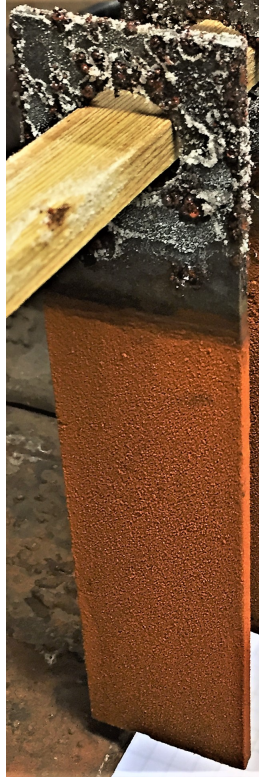
Figure 5.2: Corroded reference plate showing uniform corrosion
