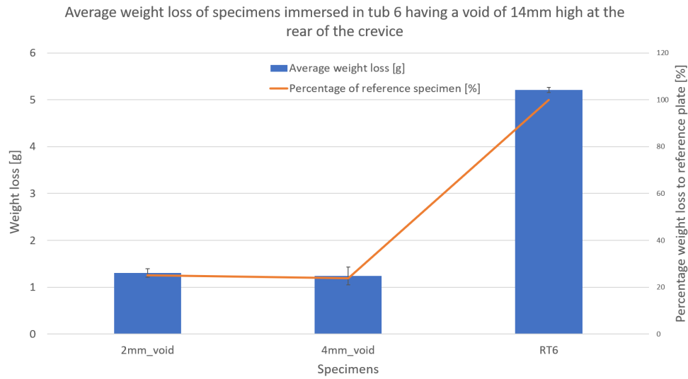
Figure 5.37: Weight loss of specimens in batch 6, having a void of 14mm high at the rear of a crevice. The weight loss of the uniform corroded reference plates is included in the plot (RT6).
