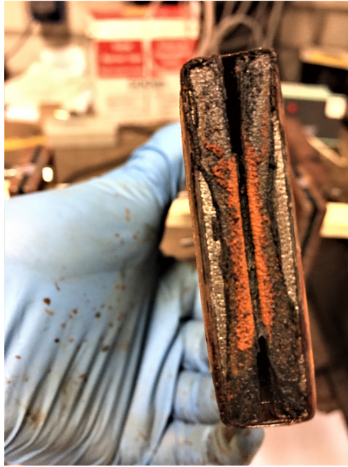
Figure 5.22: Rust forming a blockade at the mouth of a small crevice
