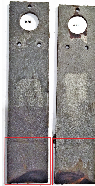
Figure 5.5: Corroded steel plate A20 and B20 of specimen S20 with a crevice of 2mm height and 50mm long. (The exposed area is indicated by the red box.)
