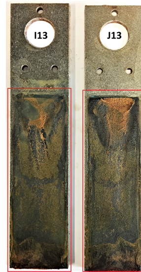
(b) Corroded steel plate I13 and J13 of specimen with a crevice of 6mm height and 150mm long. (The exposed area is indicated by the red box.)
