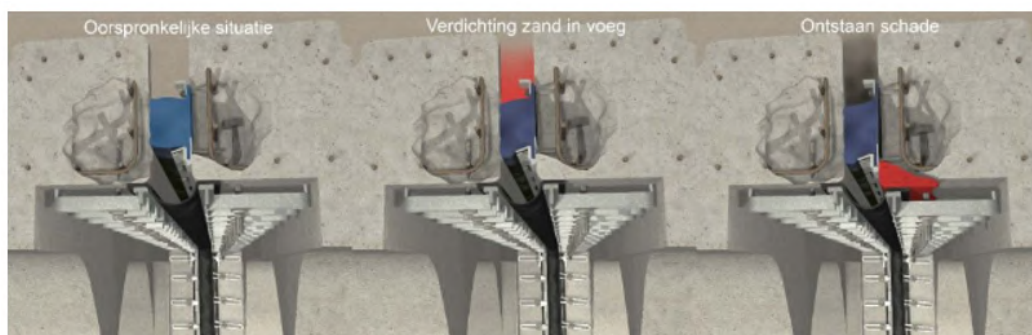
Figure 2-3: Joint movement (left), compaction of sand in joint (middle) and damage occurs (right) in Rotterdam Metro Tunnel (Molendijk et.al, 2019)
