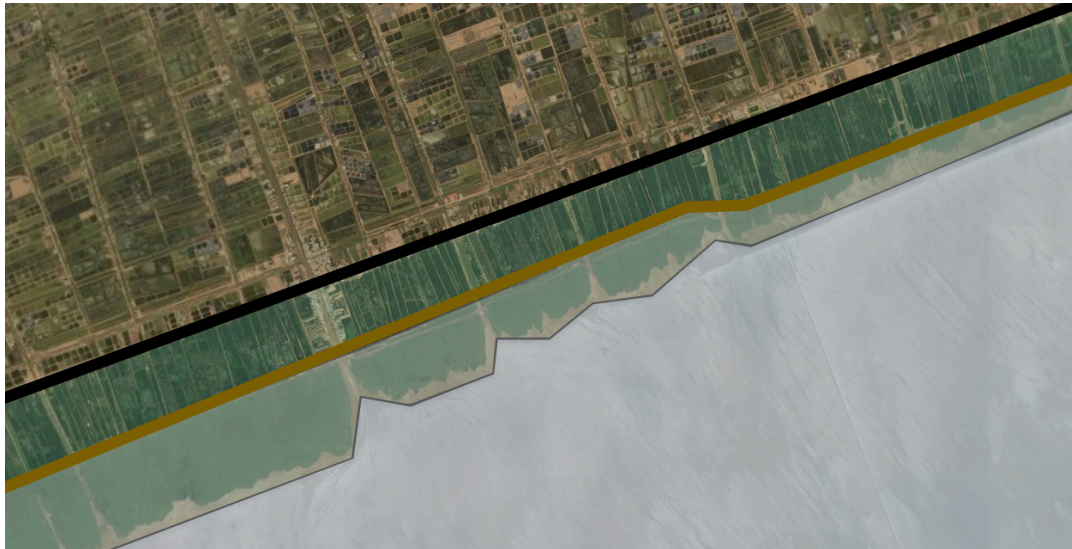
Figure 2.10: Overview of coastal land use in Bạc Liêu. The sea (light blue) borders the natural mangrove forest (light green) which is separated from the mangrove integrated fishponds (dark green) with an earthen dike (brown line). The fishponds are separated from the hinterland with a concrete dike (black line). In the hinterland, many extensive fish farms can be observed.
