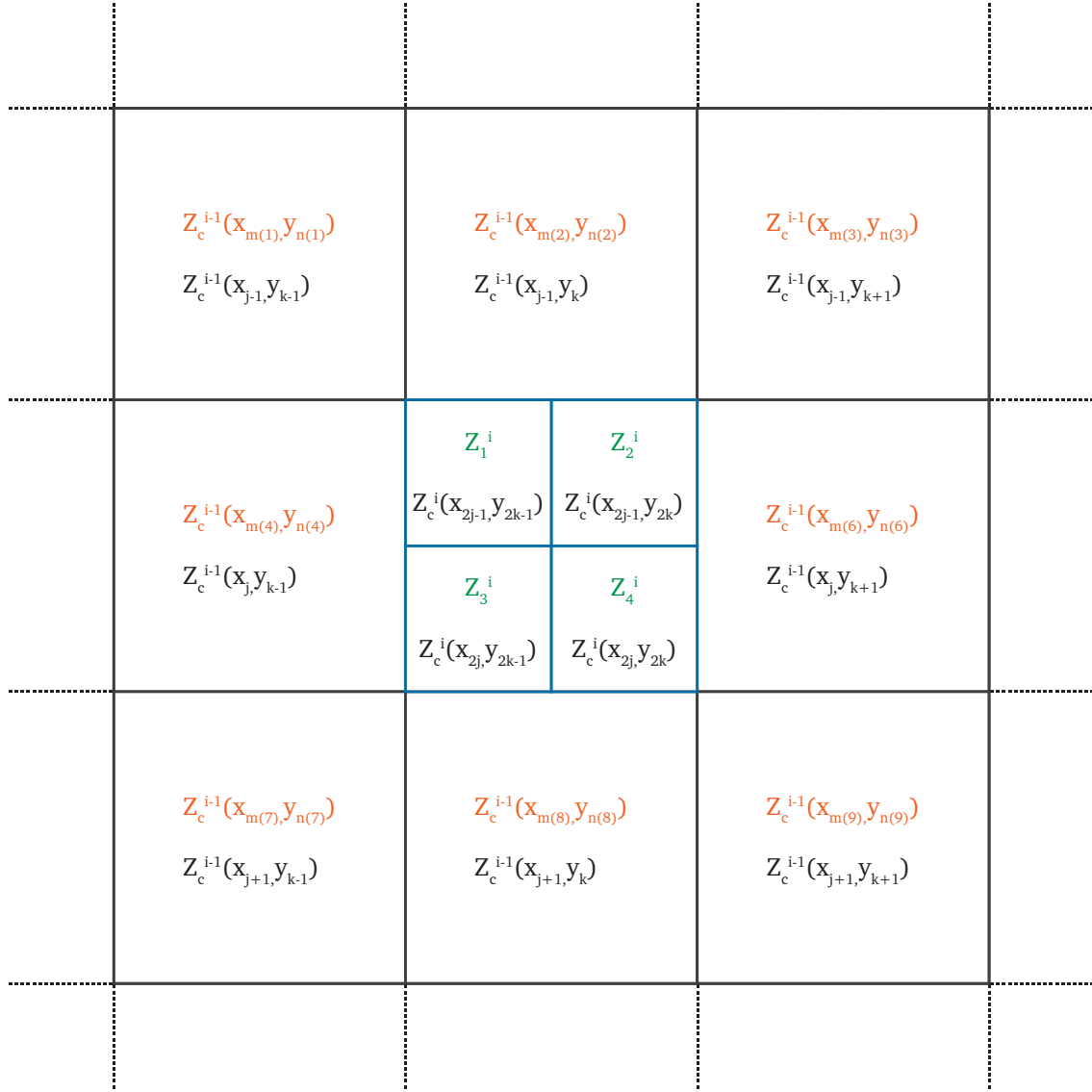
Fig. 2.12.: Numbering of cells for the LAS method in 2D where only the centre parent cell is divided in four rectangular new cells which are indicated with blue.
