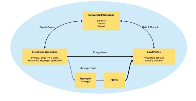
Figure 6: The CaPP system as a smart micro grid system
