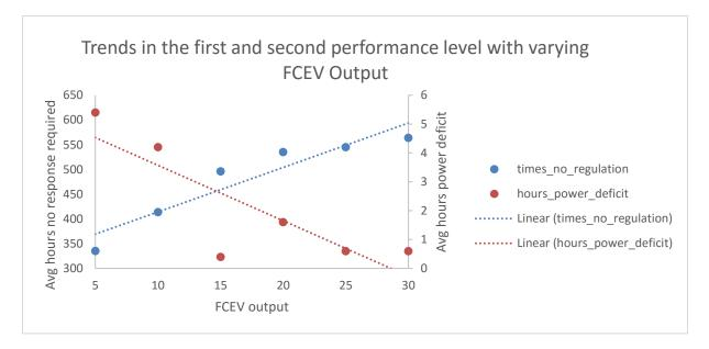
Figure 65: System performance sensitivity to FCEV output
