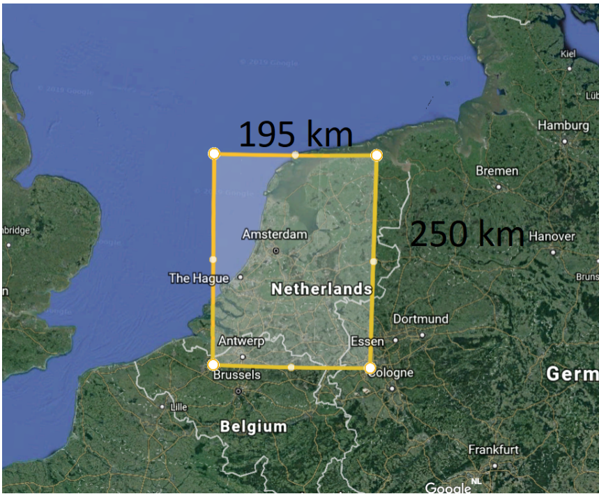
Figure 9.8: Ground coverage of FLIR tau 2 camera with 19mm lens at an altitude of 400km
