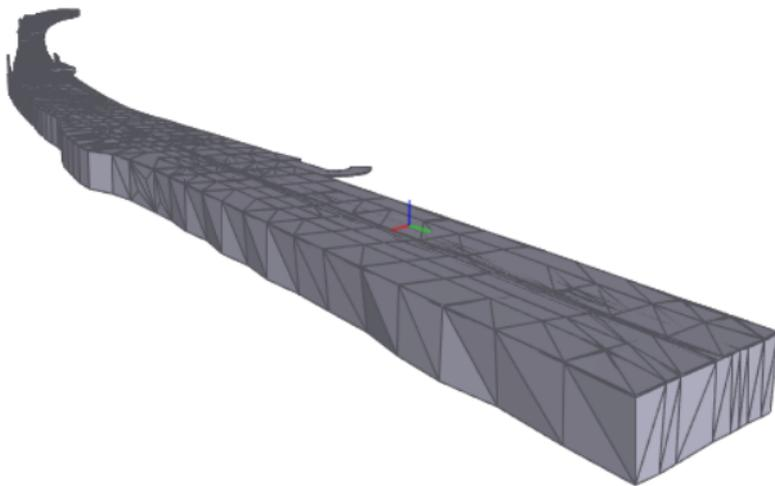
**Figure 42.** Simplified IFC model of the Heinenoordtunnel
