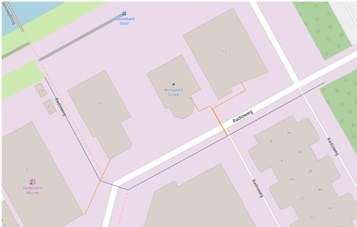
**Figure 33.** Selected pipe segments from the sewage network in Almere. Blue: main sewage pipes, orange: home connections
