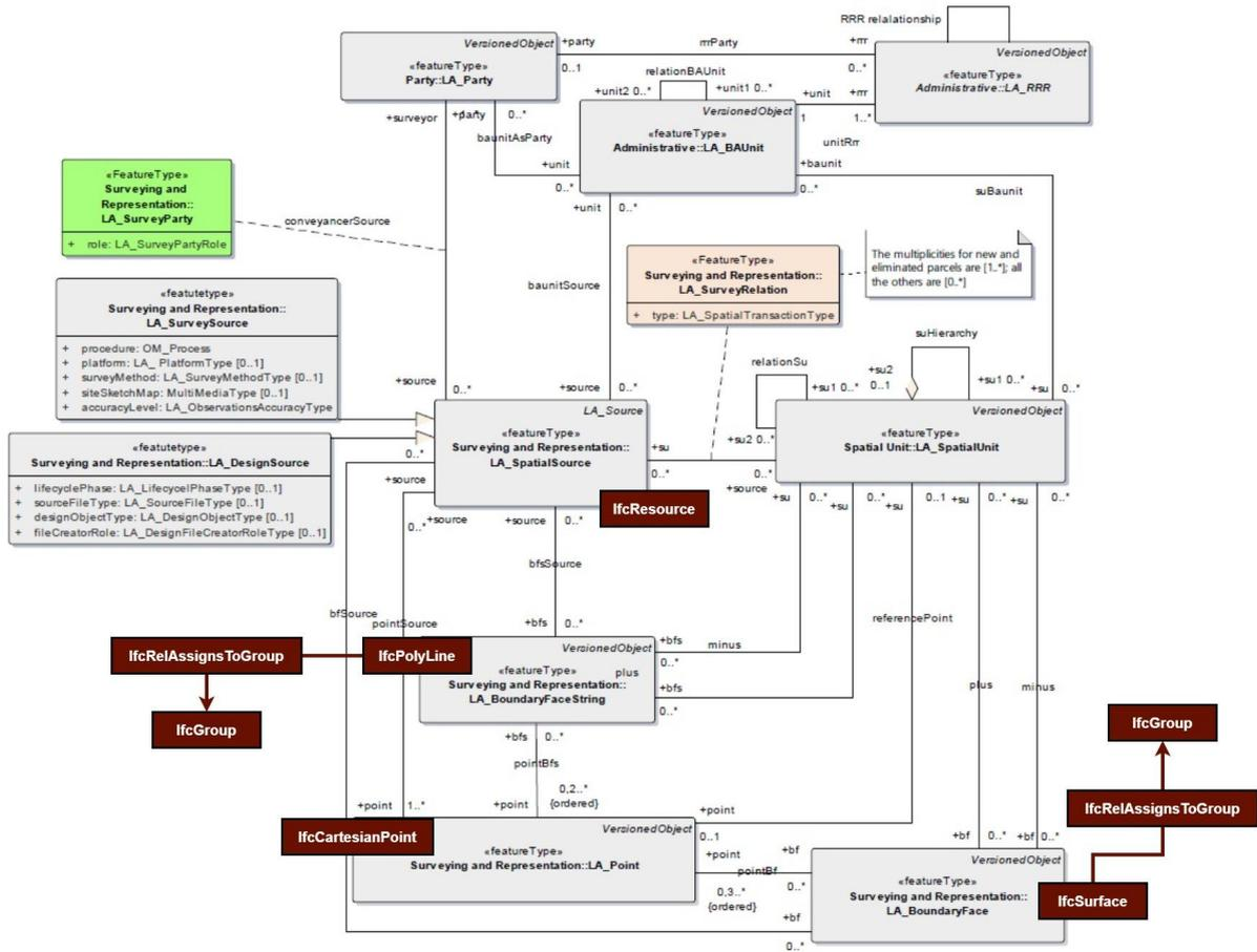
Figure 31. Mapping of the LADM classes of the Surveying and Representations subpackage to the IFC entities
