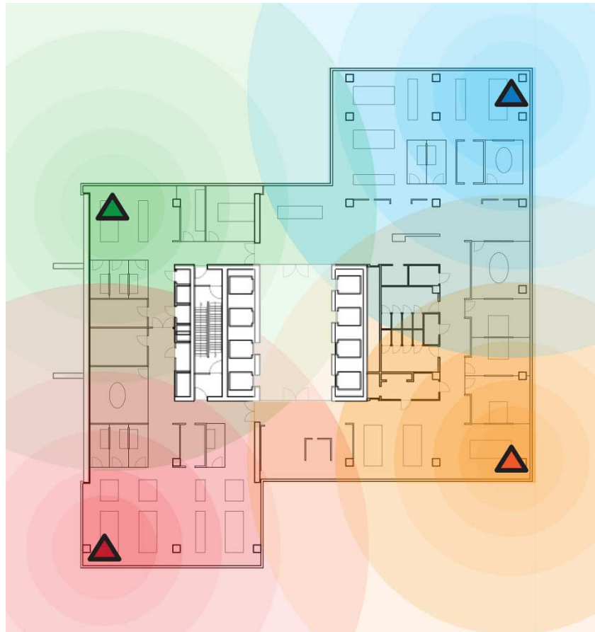
Fig.18. Concept of area rings of signal intensity per scanner – no degradation.
