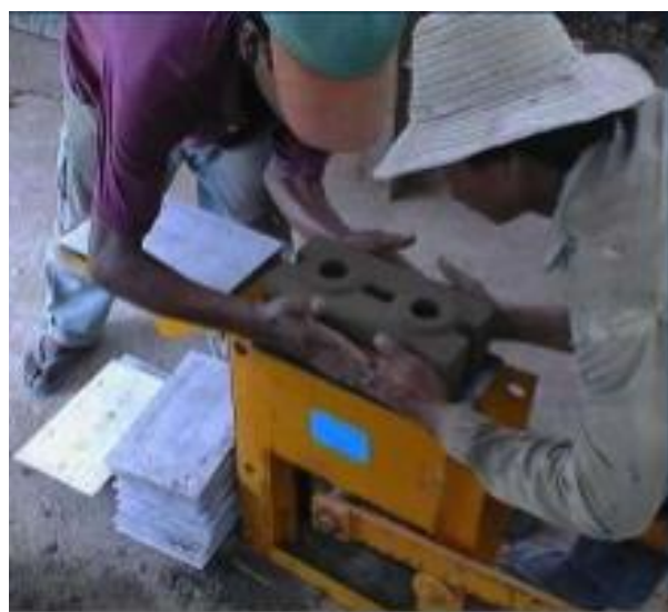
Figure 6.30. Machine used for producing interlocking bricks (Myib, 2015).
